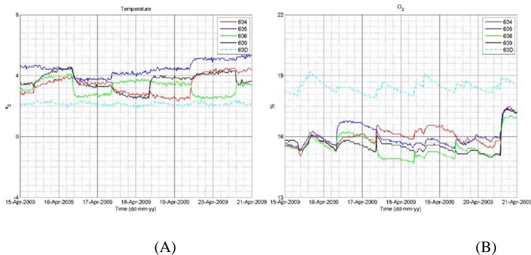
Figure 7 – Temperature and oxygen content measurements in drum no 16 and outside reference sensor (60D), for the period 15<sup>th</sup> of April to 21<sup>st</sup> of April – 2009. (A): Temperature, (B) Oxygen content
