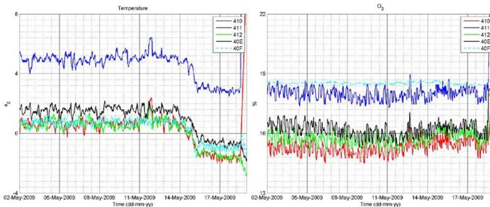
Figure 11 – Temperature and oxygen measurement for drum no 219 and outside reference sensor (40F), for the period 2<sup>nd</sup> of May to 19<sup>th</sup> of May – 2009: (A) Temperature, (B): Oxygen content.
