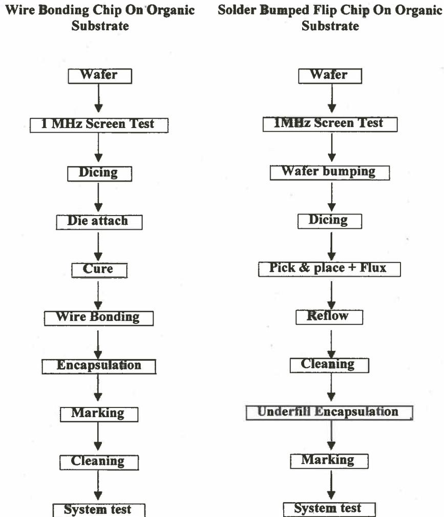
Figure 1.2 Assembly process for wire-bonding and flip-chip technologies.
