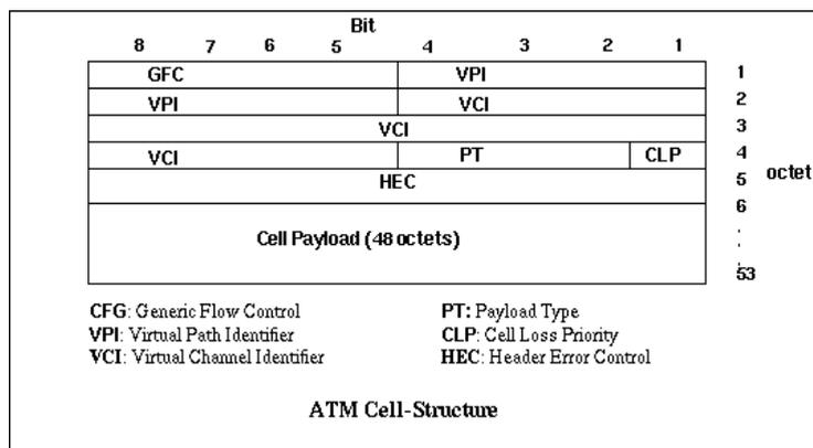
Fig. 2 ATM cell structure.
