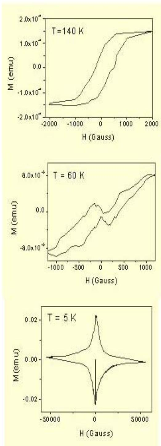
Fig. 5 Magnetization as a function of field applied parallel to the substrate-plane for  $[YBCO(100nm)/LPMO(50nm)]_2$  heterostructure recorded at three different temperatures, namely 140 K, 60 K and 5K.
