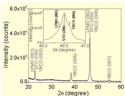
Fig. 1 XRD plot of a [YBCO(100nm)/LPMO(50nm)]<sub>2</sub> heterostructure. The inset shows the expanded plot in the 2θ range between 46 and 47°.
