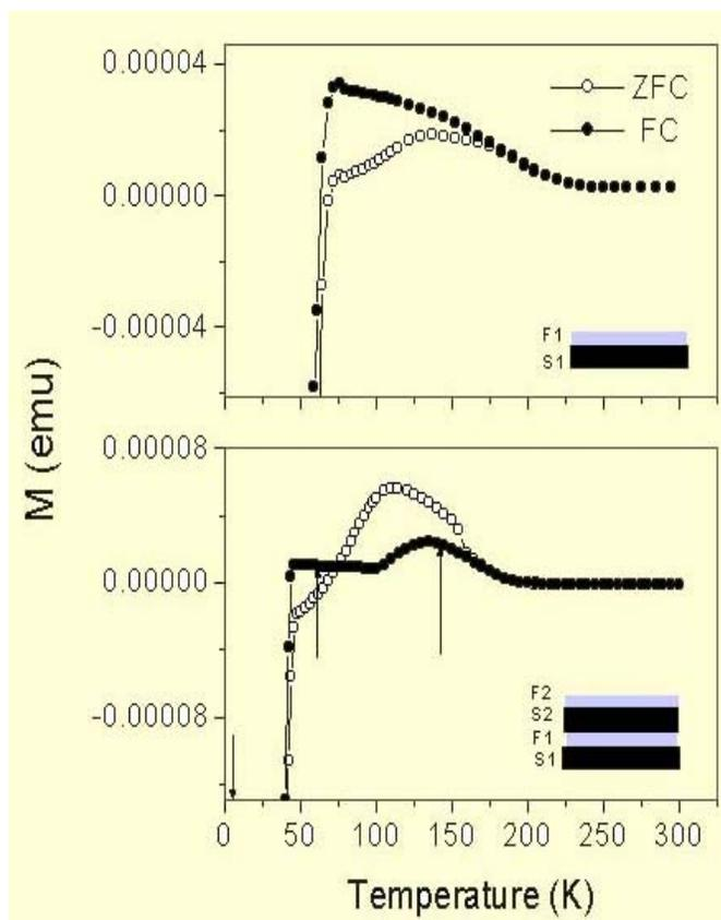
Fig. 4. Zero field cooled (ZFC) and field cooled (FC) magnetization as a function of temperature recorded for bi-layer YBCO(100nm)/LPMO(50nm) and four-layer [YBCO(100nm)/LPMO(50nm)]<sub>2</sub> heterostructures. The inset shows the schematic of the heterostructures: S1 and S2 are YBCO layers, and F1 and F2 are LPMO layers. Arrows marked at 140, 60 and 5K correspond to ferromagnetic, antiferromagnetic and diamagnetic states, respectively.
