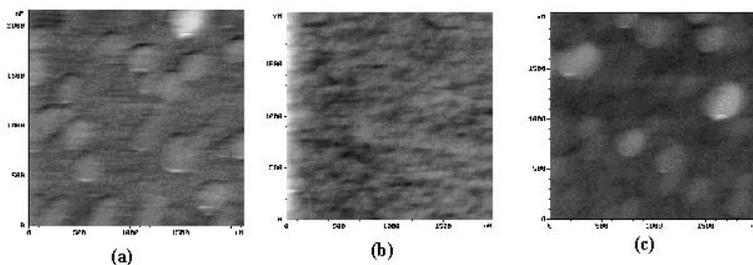
Fig. 2 2000 nm X 2000 nm AFM scans of (a) YBCO film on STO substrate, (b) LPMO film on STO substrate, and (c) YBCO(100nm)/LPMO(50nm)]<sub>2</sub> heterostructure on STO substrate.
